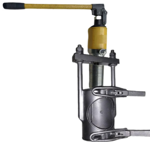
Figure 3. Elbow Cable Head Removal Tool
